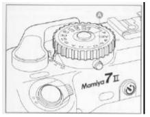
The exposure compensator functions in a number of important ways. It can be used to correct exposure values (EVs) or the differences in brightness between a primary subject and its background -especially when over or under-exposures occur. It can also be used when filters are employed or when engaged in available light photography -or under high contrast conditions (i.e. low or high key).
