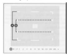
Within the viewfinder the subject area covered is indicated by the visible bright frame. Parallax is automatically compensated for according to the subject-to-lens distance. The composition will be within in the lines of the bright frame "A" for 6 x 7 format and "B" for 135 panoramic format. 83% of the field of view is visible at infinity, and 100% is visible at the minimum focusing distance. The appropriate bright frame area is automatically indexed upon lens interchange.
