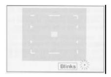
When " $\mathbf{\nabla}$ " LED blinks, it indicates overexposure. Rotate the aperture ring to stop down to a smaller f/stop until an LED indicates proper exposure.
