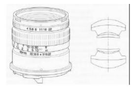
Lens construction : 6 elements in 4 groups Angle of view : 58° Minimum aperture : 22 35mm equivalent : 39mm Minimum focusing distance : 1m Magnification at minimum distance : 0.097 Area covered : 580 x 719mm Filter size : 58mm Hood : Bayonet type : 56 (L) x 67 (D)mm Dimensions Weight : 290g
