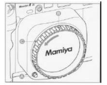
While pressing the lens release button "A" in, rotate the cap counterclockwise, and align the groove "B" on the cap's side with the lens alignment dot "C" on the body. The body cap can then be pulled out.
