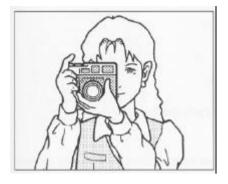
Because most out of focus pictures are the result of camera movement, make sure not to move when pressing the shutter button. Hold the camera with your elbows close to your body: pressing part of the camera on your forehead will help stabilize it. Then gently release the shutter.
