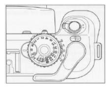
When taking an exposure longer than 4 seconds, set shutter to "**B**" (bulb). At "**B**" the shutter will remain open as long as the release is pressed down.
