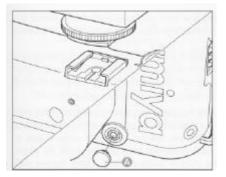
The Mamiya 7II features an X synchro flash terminal and its lens shutter system permits flash synchronization at all shutter speeds.
