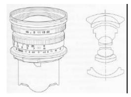
Lens construction : 10 elements in 6 groups : 92° Angle of view Minimum aperture : 22 35mm equivalent : 21mm Minimum focusing distance : 1m Magnification at minimum distance : 0.049 Area covered : 1145 x 1421 mm Filter size : 67mm Hood : Bayonet type : 42 (L) x 72 (D)mm Dimensions Weiaht : 390g
