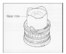
4) When mounting the 43mm, 50mm and 65mm wide angle lenses make sure that the rear lens rims do not touch the rangefinder coupling roller.
