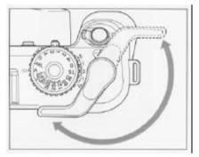
After completing the last exposure, wind the advance lever several times until the film with its backing paper is completely wound onto the take-up spool. The advance lever will become easier to actuate when the film has been completely wound on the spool.
