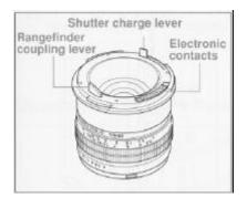
3) Be careful not to damage the rangefinder coupling lever and the shutter cocking lever at the rear of each lens.
