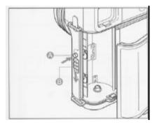
While depressing the back cover lock button "A", simultaneously push down the lock lever "B" in the direction of the arrow and the back will open. When closing the back cover, securely press both corners until it clicks.
