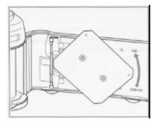
This camera can use either 120 or 220/135 film. To set for the type of film used, simply rotate the pressure plate in either direction of the arrow until the white dot is at 120" or "220/135".
