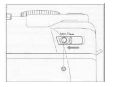
While pressing the lock release button "A", move the lever in the arrow direction to the multiple exposure position.
