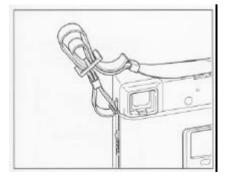
Pass the neck strap through the carrying strap lugs, and fasten it as shown.
