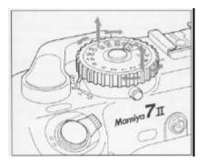
Set the film speed of the film being used by lifting up the outer rim of the shutter speed dial and rotate it until the correct ISO value appears in the window. \*Be sure to set the exact film speed, as otherwise incorrect exposure will result.
